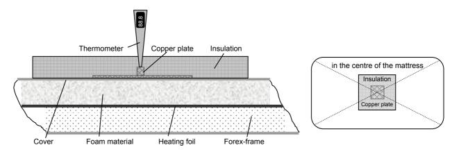
The temperature, measured on the copper plate between the mattress surface and the insulation layer must be:  $37.0^{\circ}C \pm 0.5^{\circ}C$ .
