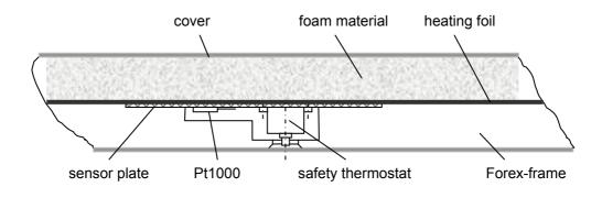
The temperature between the heating foil and sponge material (heating temperature) is measured and controlled. The display shows the temperature calculated between the child and the cover.
